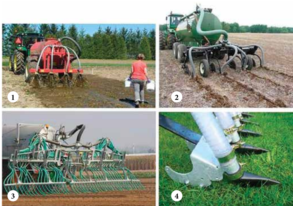
Figure 32. Four methods of introducing the substrate into the soil: application to surface with spray splashing (1), subsoil application (2), with filling from hoses (3) and trailer colter (4)
